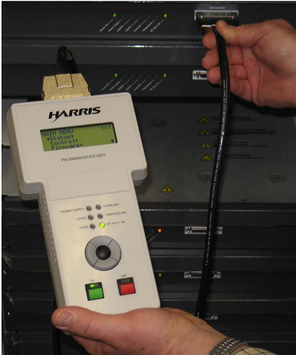
Figure 1-2 PA Diagnostics Unit and Cable
