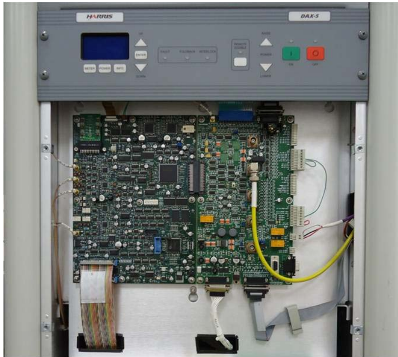
Figure 2-1 DAX5 Front View With Access Panel Removed Showing Interconnection of RF and Audio I/O
